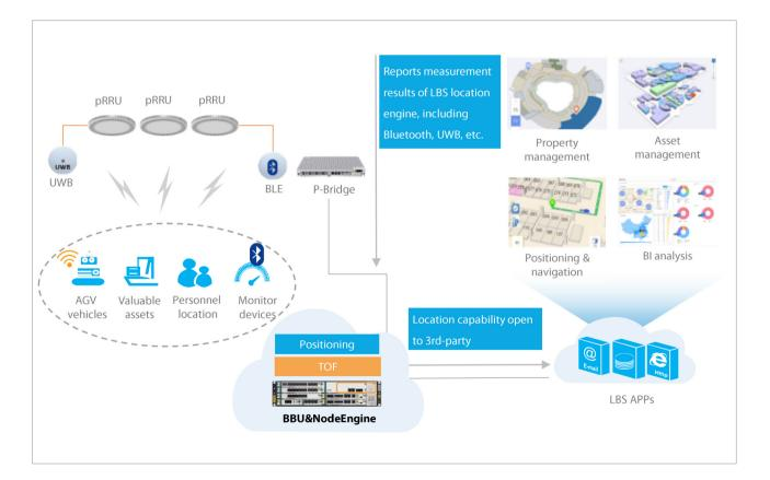
Figure 4-16 Open positioning capability
